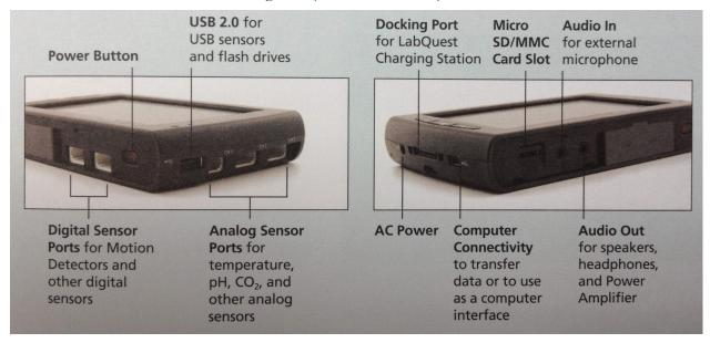
The photo on the right shows the AC power connection used to charge the battery and to run the device under AC power. The mini USB port provides a means for connecting the device to a computer, which you can use to transfer data from the LabQuest 2 to your computer, or use to operate the device from your computer (more on both topics later).
