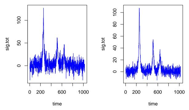
Figure on the left is a single scan. Figure on the right is the sum of four scans.
