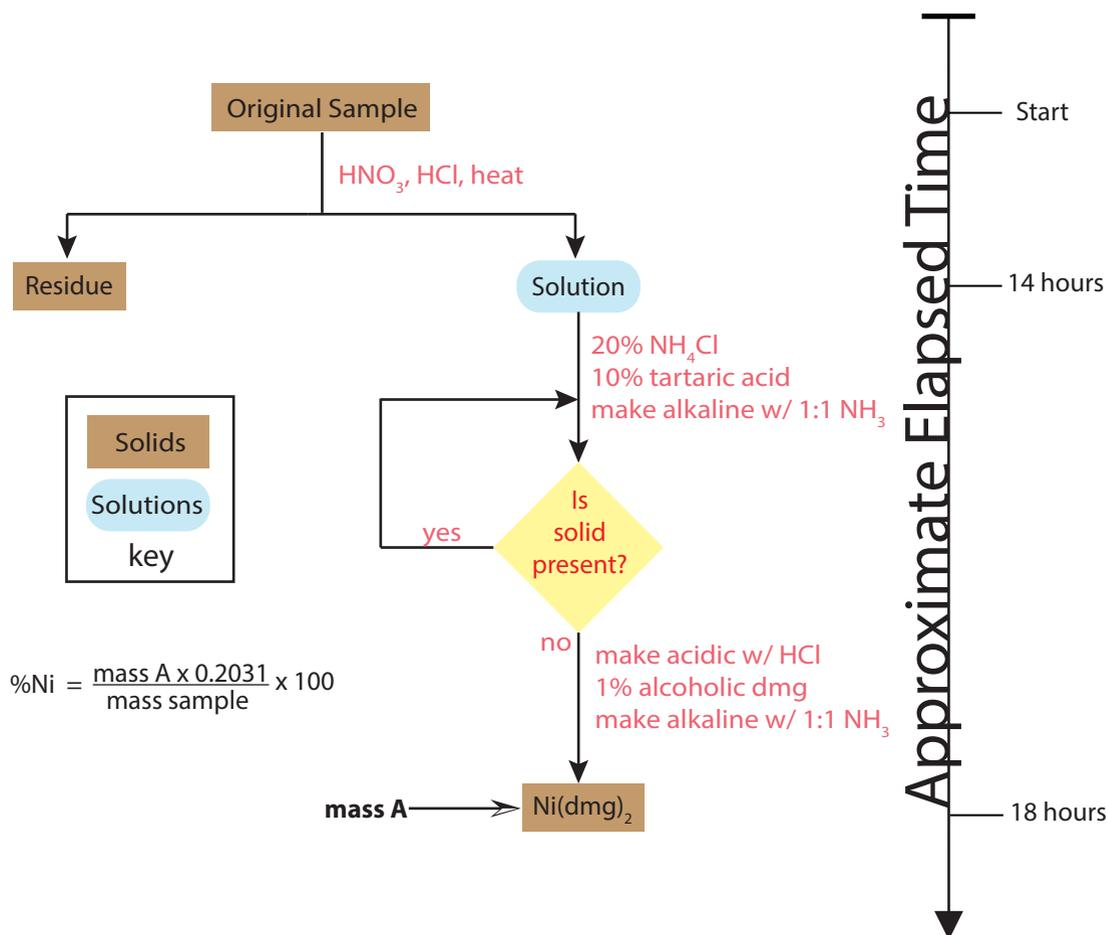
**Figure 1.2** Gravimetric analysis for Ni in ores by precipitating  $\text{Ni}(\text{dmg})_2$ . The timeline shows that it takes approximately 18 hours to analyze a single sample, substantially less than 58 hours for the method in Figure 1.1. The factor of 0.2301 in the equation for %Ni accounts for the difference in the formula weights of Ni and  $\text{Ni}(\text{dmg})_2$ ; see Chapter 8 for further details.
