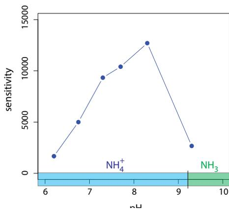
**Figure SM11.10** The sensitivity of an amperometric biosensor for  $\text{NH}_4^+$  over the pH range 6.2 to 9.3. Superimposed on the x-axis is a ladder diagram for  $\text{NH}_4^+$ , which shows its weak acid form in **blue** and its weak base form in **green**.
