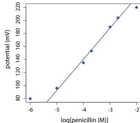
**Figure SM11.2** Calibration data (blue dots) and calibration curve (blue line) for the data in Problem 10. The calibration curve is restricted to  $\log[\text{penicillin}]$  values between  $-2.70$  and  $-5.00$ .
