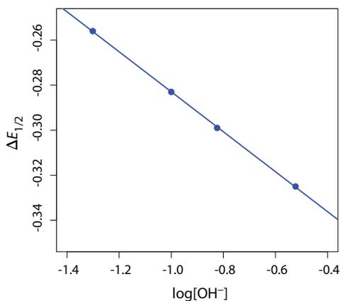
**Figure SM11.13** Data (blue dots) and regression line (blue line) for Problem 37 used to determine the stoichiometry and the formation constant for a complex between  $\text{Pb}^{2+}$  and  $\text{OH}^-$ .
