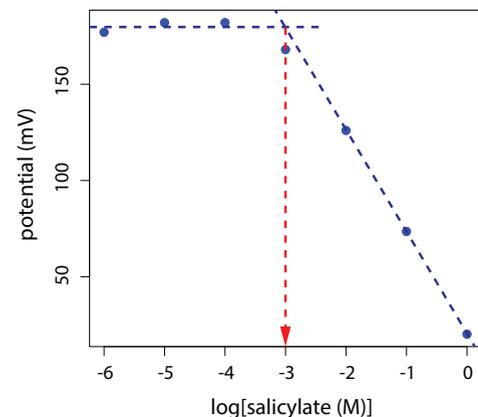
**Figure SM11.1** Potential versus concentration data for a salicylate ion-selective electrode in the presence of 0.1 M benzoate. The blue dots are the data from Problem 5 and the blue dashed lines show the regions where the ISE's potential is determined by the concentration of benzoate or of salicylate. The red dashed line shows the concentration of salicylate that yields the same potential as does 0.1 M benzoate.
