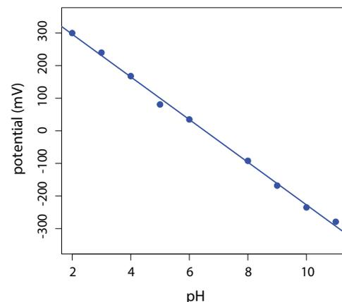
**Figure SM11.4** Calibration data (blue dots) and calibration curve (blue line) for the data in Problem 12.
