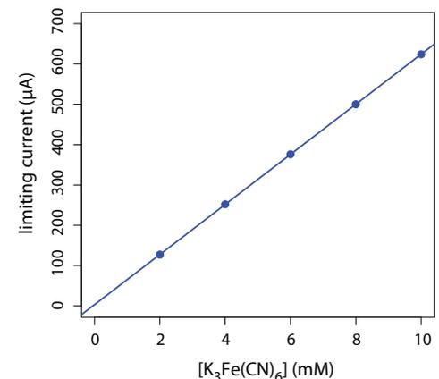
Figure SM11.7 Calibration data (blue dots) and calibration curve (blue line) for the data in Problem 23.
