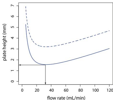
**Figure SM12.2** The van Deemter plot for Problem 7d. The solid blue line shows the plate height as a function of flow rate for an open-tubular column and the dashed blue line is for the packed column in Problem 7a. The arrows identify the optimum flow rate of 33 mL/min with a plate height of 1.56 mm.
