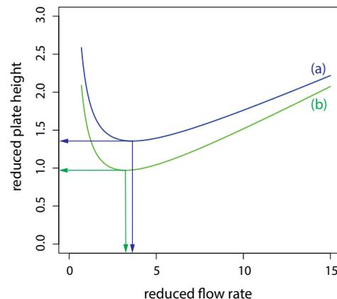
**Figure SM12.3** The van Deemter plot for Problem 8a. The solid blue line shows results for the first row of data and the solid green line shows the results for the last row of data. The arrows identify the optimum reduced flow rate and the optimum reduced plate height for each set of data.
