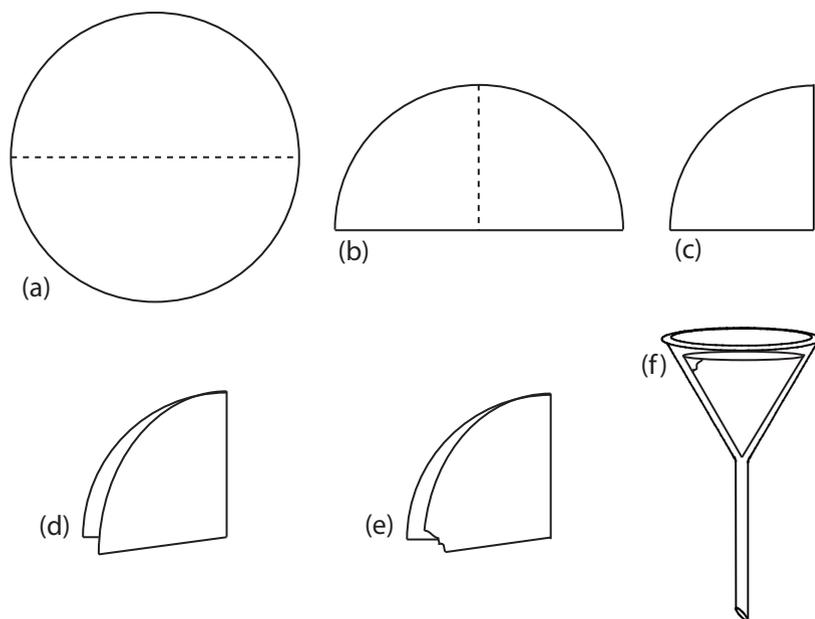
**Figure 8.7** Preparing a filter paper cone. The filter paper circle in (a) is folded in half (b), and folded in half again (c). The folded filter paper is parted (d) and a small corner is torn off (e). The filter paper is opened up into a cone and placed in the funnel (f).
