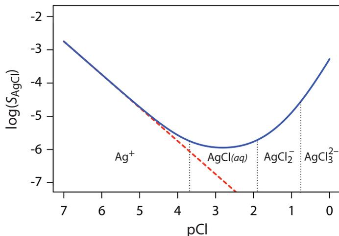
**Figure 8.1** Solubility of AgCl as a function of pCl. The dashed red line shows our prediction for  $S_{\text{AgCl}}$  if we incorrectly assume that only [reaction 8.1](#) and equation 8.2 affect silver chloride's solubility. The solid blue curve is calculated using equation 8.7, which accounts for [reaction 8.1](#) and reactions 8.3–8.5. Because the solubility of AgCl spans several orders of magnitude,  $S_{\text{AgCl}}$  is displayed on the  $y$ -axis in logarithmic form.
