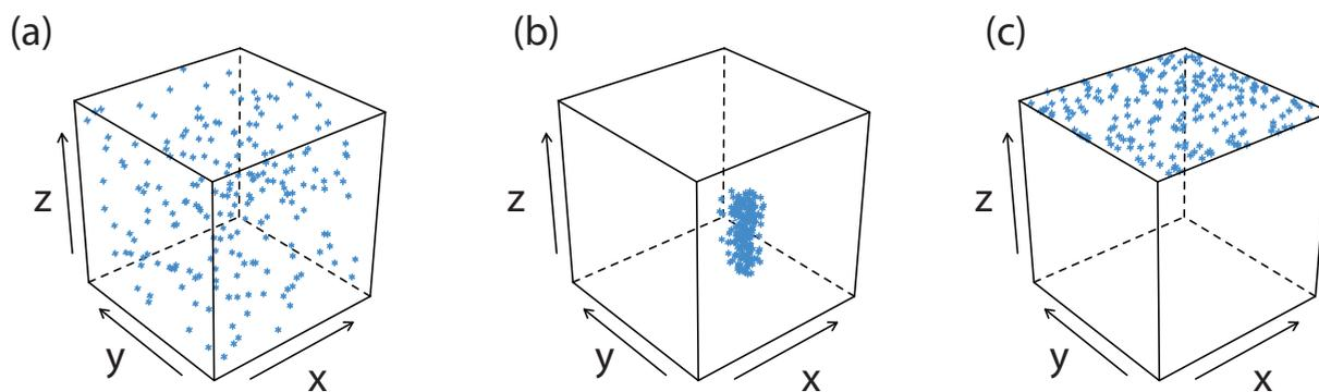
**Figure 8.4** Three examples of impurities that may form during precipitation. The cubic frame represents the precipitate and the blue marks are impurities: (a) inclusions, (b) occlusions, and (c) surface adsorbates. Inclusions are randomly distributed throughout the precipitate. Occlusions are localized within the interior of the precipitate and surface adsorbates are localized on the precipitate's exterior. For ease of viewing, in (c) adsorption is shown on only one surface.
