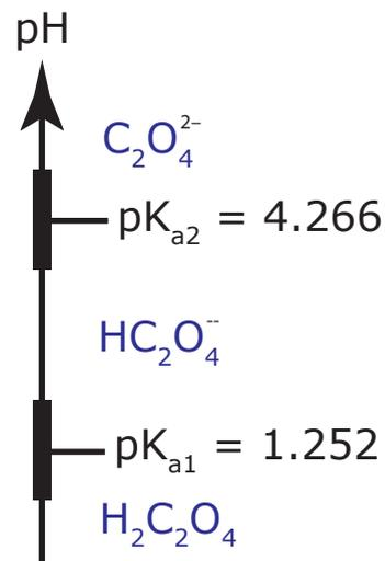
**Figure 8.17** pH ladder diagram for oxalic acid,  $\text{H}_2\text{C}_2\text{O}_4$ .
