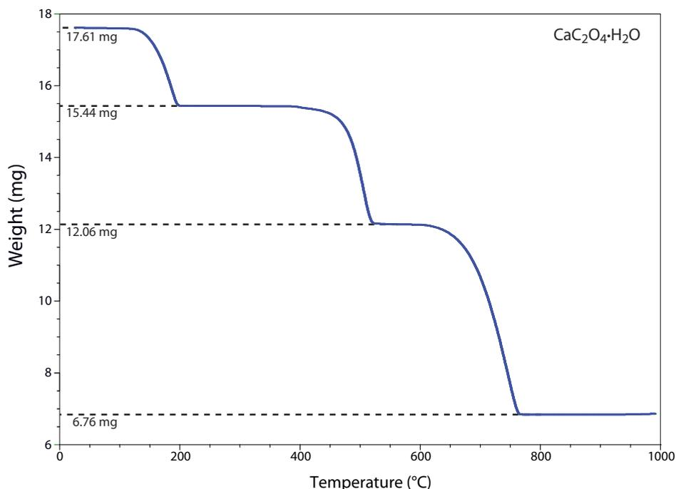
**Figure 8.10** Thermogram for  $\text{CaC}_2\text{O}_4 \cdot \text{H}_2\text{O}$  obtained by heating a sample from room temperature to  $1000^\circ\text{C}$  at a rate of  $20^\circ\text{C}/\text{min}$ . Each change in mass results from the loss of a volatile product. The sample’s initial mass and its mass after each loss are shown by the dotted lines. See Example 8.4 for information on interpreting this thermogram.
